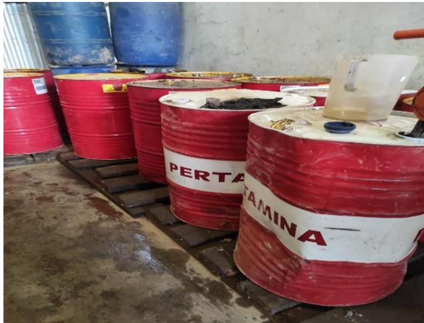
Photo 12: Chemical drum storage area, lacking in appropriate labelling, with stained floor (PT DWT)
