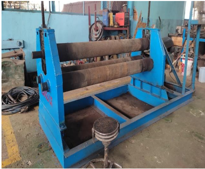
Photo 11: Roll Plate Machine, lacking in machine guarding (PT BAS)
